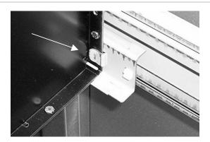
The suspension slide inner members have a cut out slot for the rear of the drawer to fit into. (In most instances it is not possible to see behind the drawer to view whether the drawer has located properly, but sometimes will this be apparent when the front of the drawer has been fitted, as the drawer will not travel smoothly or align correctly when closed).
